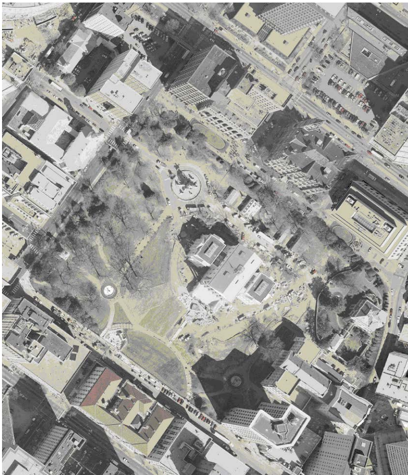
Figure 3-C.6. Example of a DOQQ: Virginia State Capitol Campus Source: Virginia Base Mapping Program
