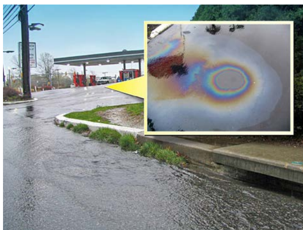
Figure 4.34. Fueling Stations Can Be Stormwater Hotspots Source: Chesapeake Bay Stormwater Training Partnership
