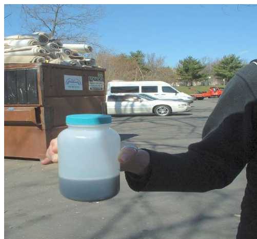
Figure 5-D.23. Sample of Illicit Discharge From a Storm Drainage Pipe Outlet
