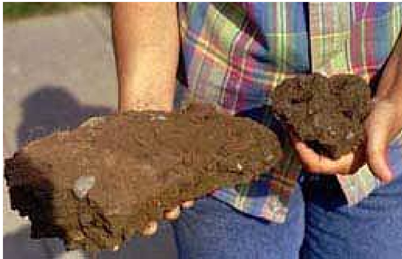
Figure 5-C.9. Compacted Urban Soil
