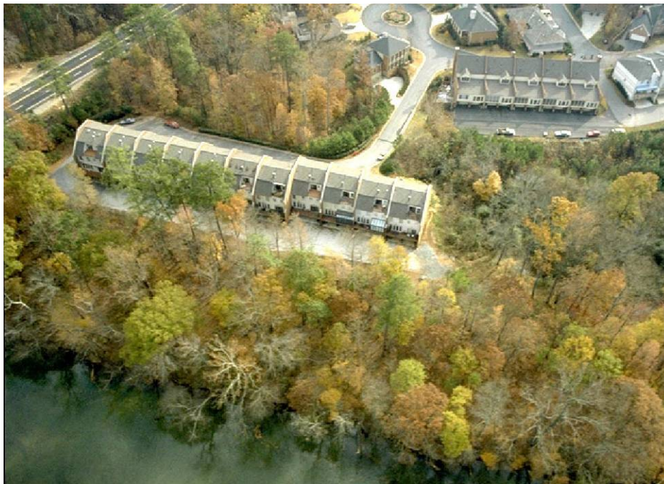
Figure 6.41. Example of Site Footprinting
