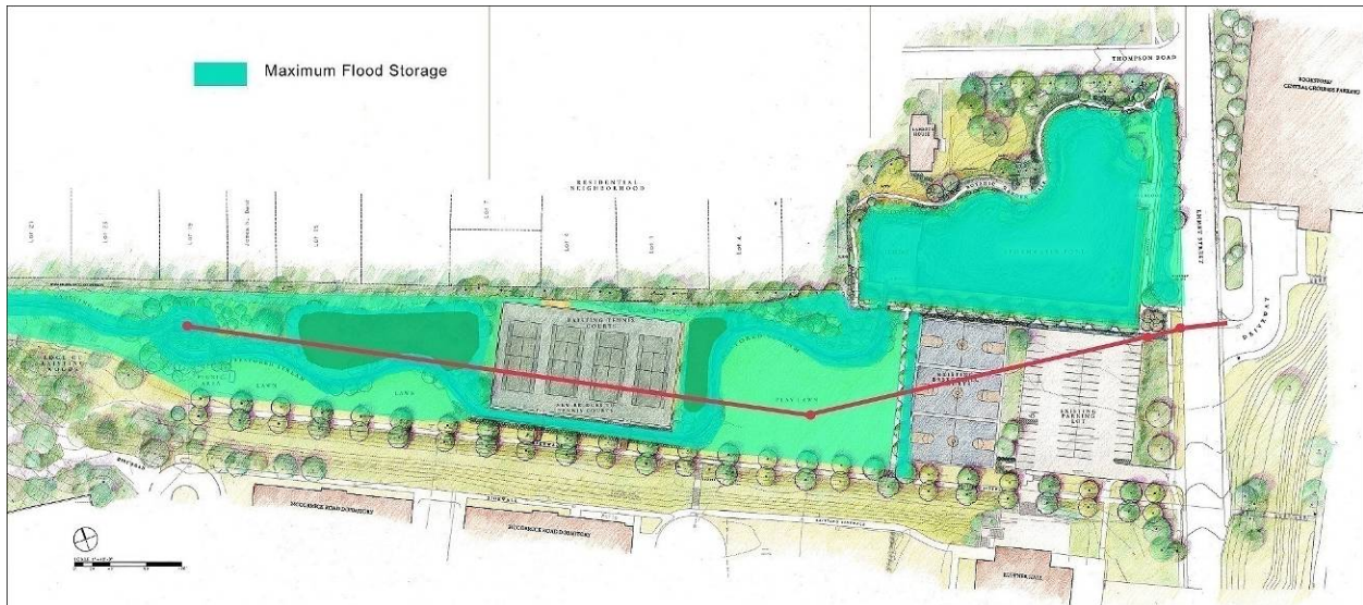
Figure 6.108. UVA Dell Project Site. Location of Rain Gardens and the Maximum Flood Zone. Source: Nelson Byrd Woltz Landscape Architects
