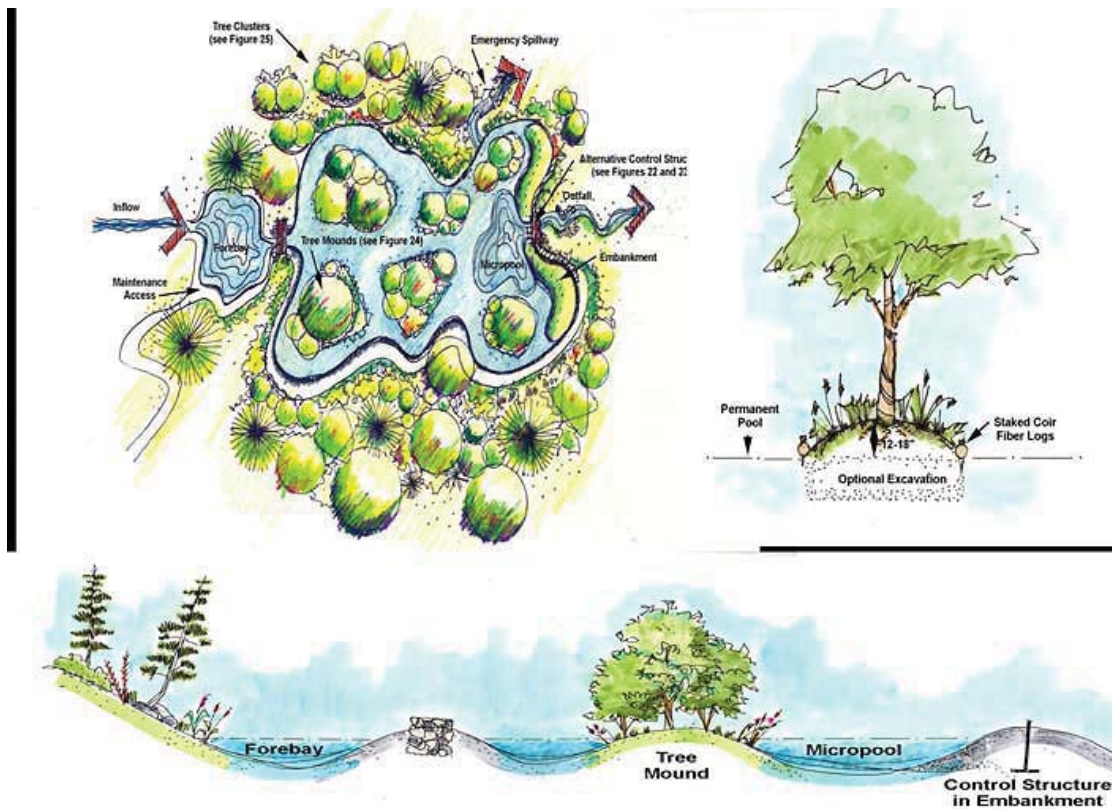
Figure 7.18. Wooded wetlands are a preferred stormwater treatment option for crossing retrofits Source: CWP, 2007
