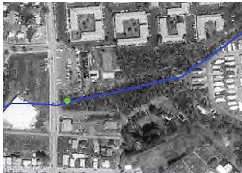
Figure 7.19. Crossing retrofits are easy to find when road network and drainage layers are superimposed Source: CWP, 2007
