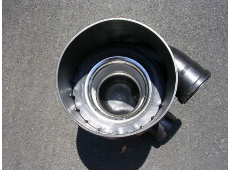
Figure 6.10. Interior of Vortex Filter
