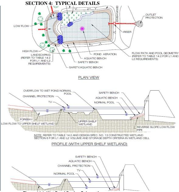
Figure 14.1. Wet Pond Design Schematics
