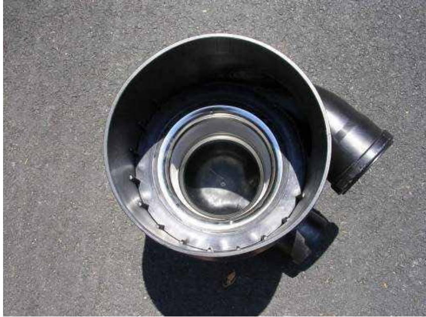
Figure 6.9. Interior of Vortex Filter
