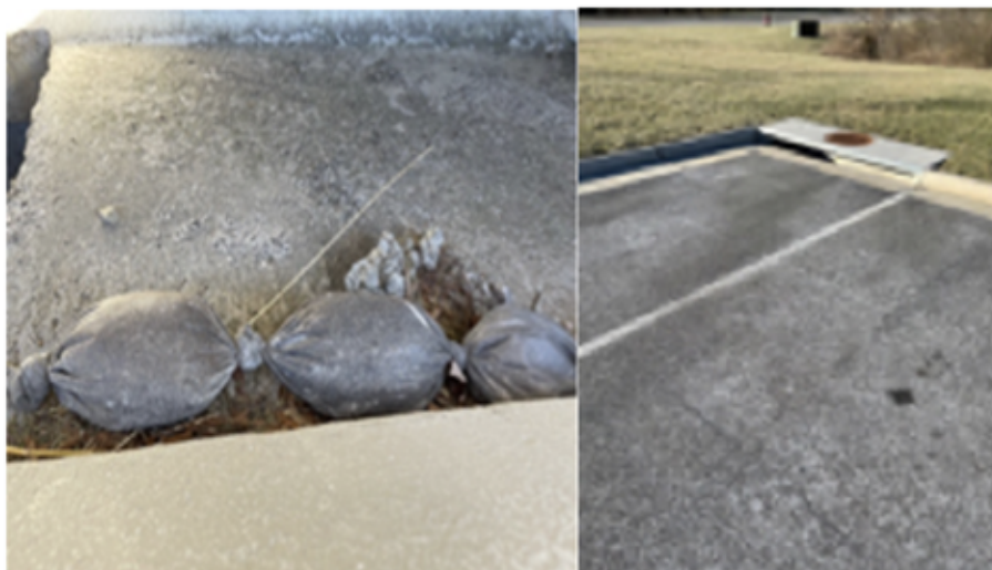
Figure 31. Containment “socks” (Left) were placed in or around parking lot drains (Right) to filter surface runoff and keep sodium, chloride, or other ions out of the environment. Knots in the sock fabric isolate different fillers that have high ion binding capacity in this experimental system.
