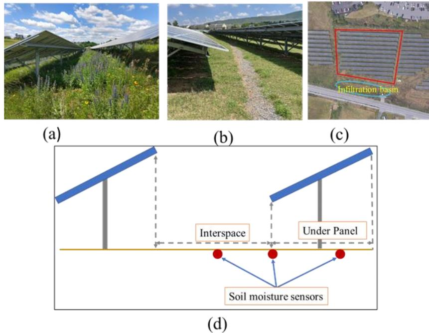
**Figure 5.** Photos and schematic of the studied solar farms: (a) solar farm 1 (steep site); (b) solar farm 2 with infiltration trench; (c) infiltration basin at base of solar farm 1, and (d) schematic of key monitoring locations relative to solar panels.
