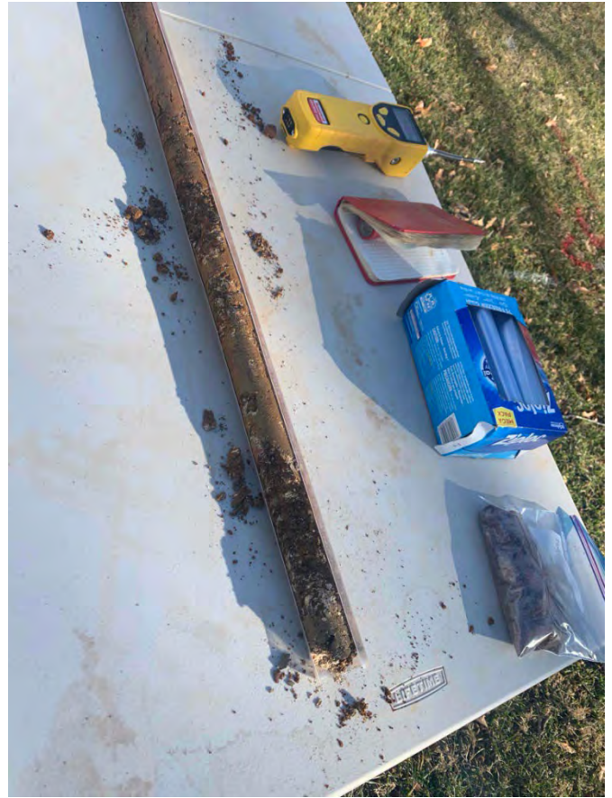
14. Collection of soil samples via new clear, thin walled, PVC liners (12/22/2023)
