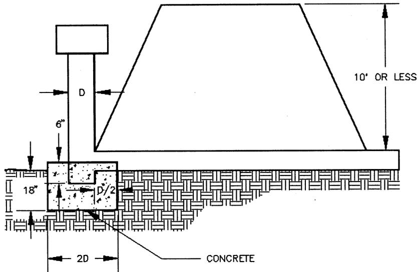
STEEL BASE FOR EMBANKMENT 10' OR LESS IN HEIGHT
