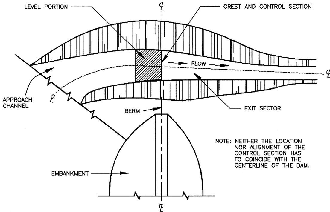
NOTE: NEITHER THE LOCATION NOR ALIGNMENT OF THE CONTROL SECTION HAS TO COINCIDE WITH THE CENTERLINE OF THE DAM.
