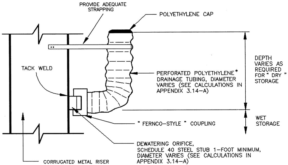
NOTE: WITH CONCRETE RISER, USE PVC SCHEDULE 40 STUB FOR DEWATERING ORIFICE
