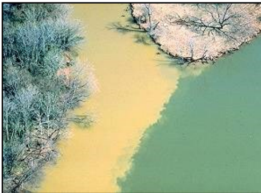
Figure 14: A Sediment Plume Entering a River
