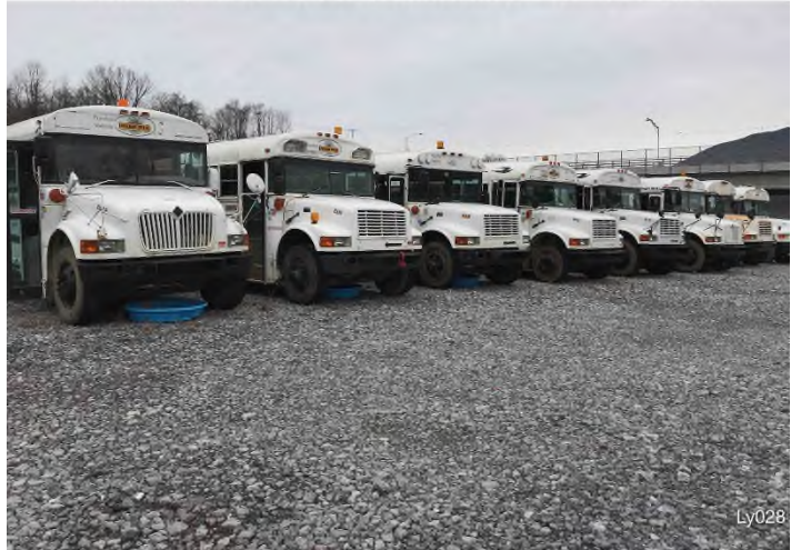
Fig. 4: Laydown Yard 028 – Secondary containment placed under equipment storage to contain potential leaks.
