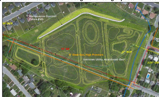
Figure 7.6. Photo showing constructed wetland retrofit design for existing dry detention basin
