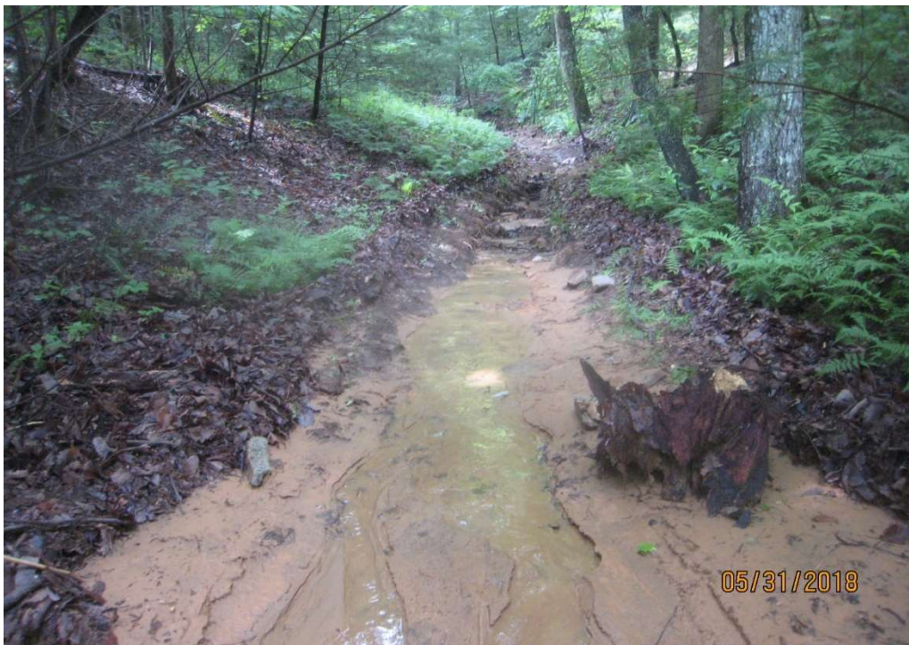
Sediment within channel ~685-feet from MVP LOD Channel 3 to 5-feet wide; Sediment depth 3-inches in thalweg, 3 to 6-inches on sediment bars
