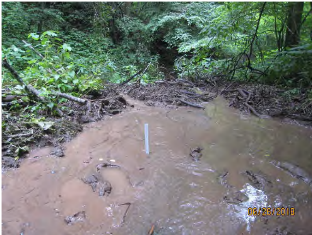
Photo 2: 4.5' of sediment at debris dam ~210' from Photo 1
