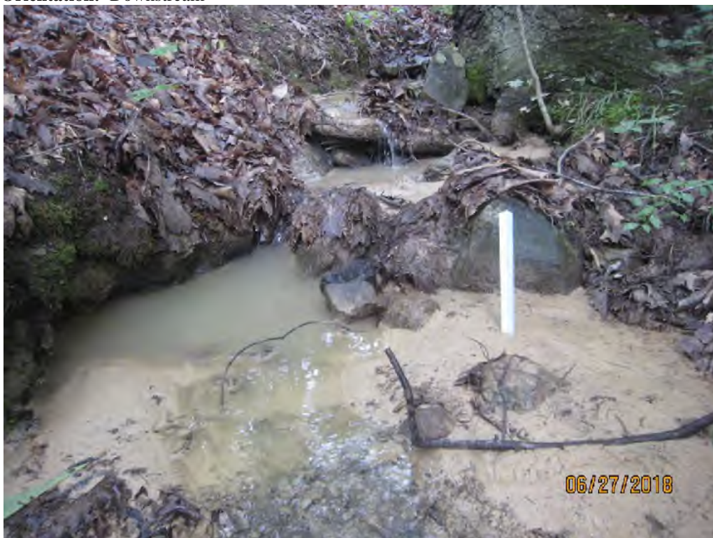
Photo 2: Sediment in stream ~685' from LOD; Depth = 3" Orientation: Upstream
