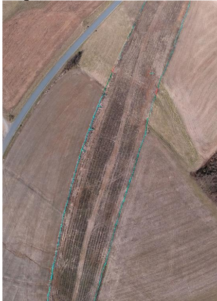
Photo 5. MVW Photo Jan.14, 2021 of MP 293.1 showing adequate vegetative stabilization.
