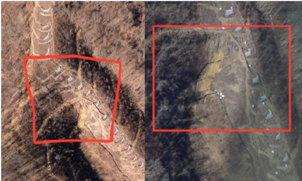
Photo 11. MVW photo soil slip. MVP has stabilized this area and is currently working on a plan to remedy the slip.
